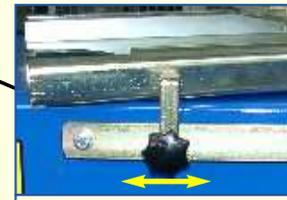
A considerable detail is the rotation stop (limit stop). This is arranged in such a way that the grinding wheel always remains within the grinding area and doesn't grind over the edge, neither at the beginning, nor at the end of the blade.
